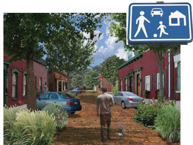
Rendering of a woonerf, or living street where pedestrians and cyclists have legal priority over motorists from hamercenter.psu.edu
