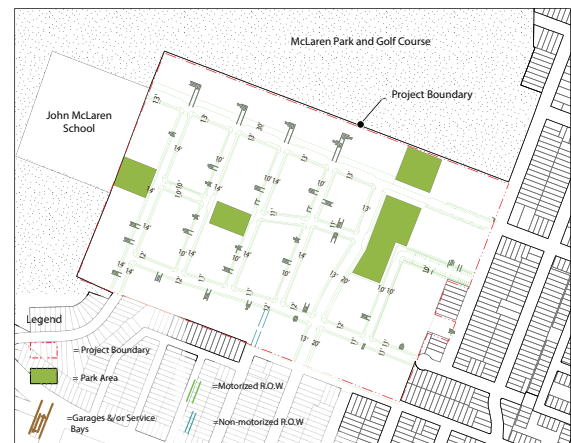
A stage 1 LEED-ND project map showing the spatial location of garages and service bays for compliance with Walkable Streets prerequisite 1, part d
