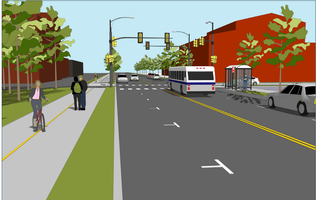
Rendering of Pine Street perspective showing separated multi-modal path, bus shelters, pedestrian crossings and stop lights
